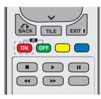
2 If you press the left/right buttons or press the ON button repeatedly, the Picture ID cycles through OFF and 0 to 4. Assign the ID you want.
